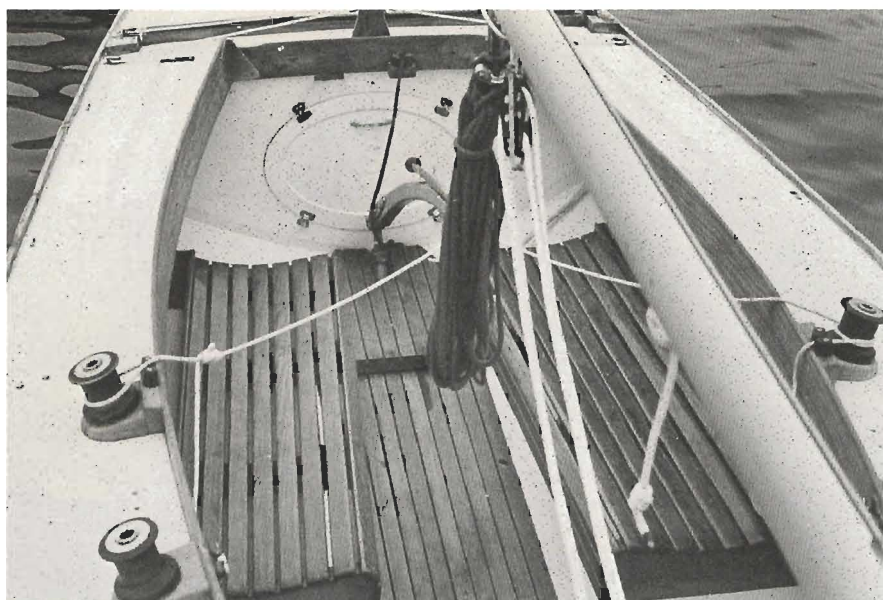
The aft end of the Shields cockpit, with wide seats, traveler control lines led forward below the deck, and mid-boom "headknocker" mainsheet cleat.
