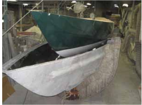
Removing the Boat from the Hull Mold
